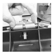
4. Slide the lockwasher (P/N 10062951) over the latch-spring "legs".
