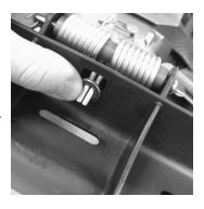
Lift the latch-spring "legs" slightly with a prybar or channel locks.
