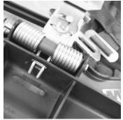
Slide the latch-springs together. Note: Sliding the latch-springs together may require the use of both hands or pliers.
